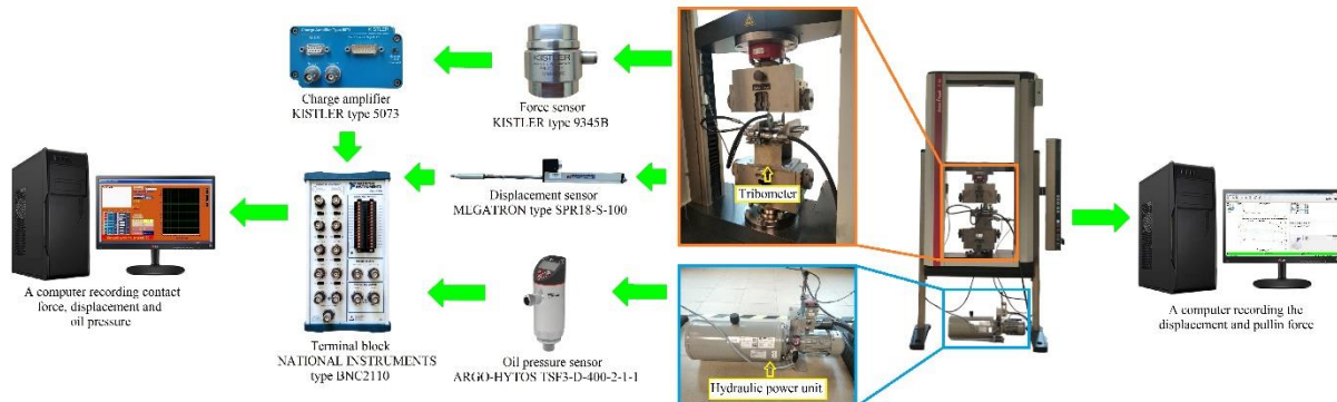
Fig. 5. Diagram of the research stand.
