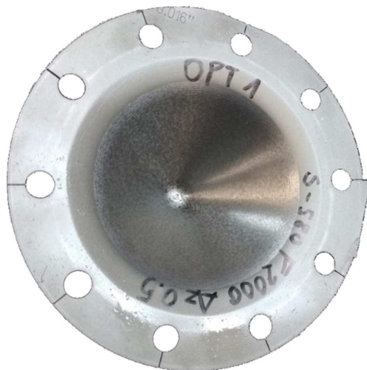
Fig. 5. Successfully achieved the drawpiece using optimized parameters
