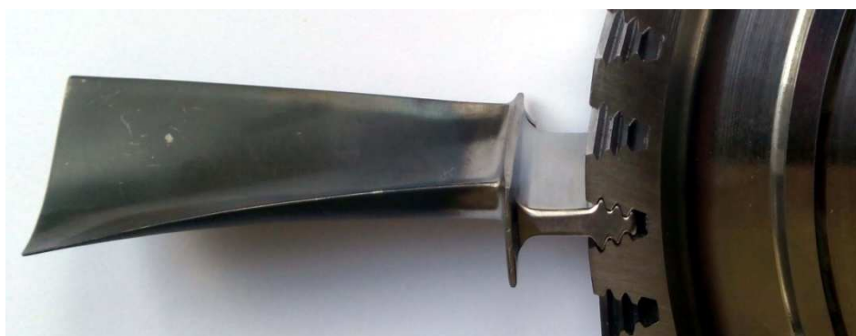
Fig. 1. View of the turbine blade and the fragment of the disc with fir tree slots
