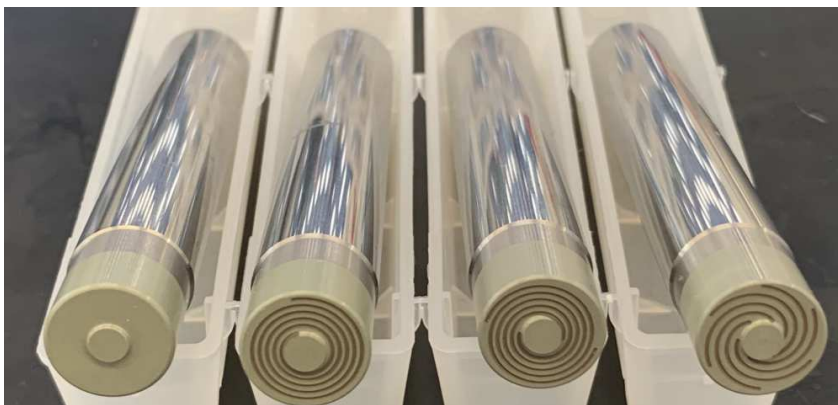
Fig. 3. Different type of shoulder profile of FSW tools with and without groves
