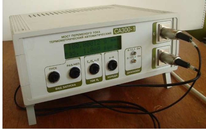
Fig. 2. Automatic bridge AC type CA 300
