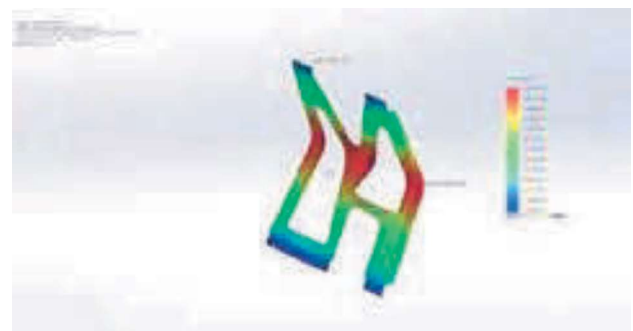
Fig. 13. Beam 3. Stress distribution (Huber-Mises) and displacement
