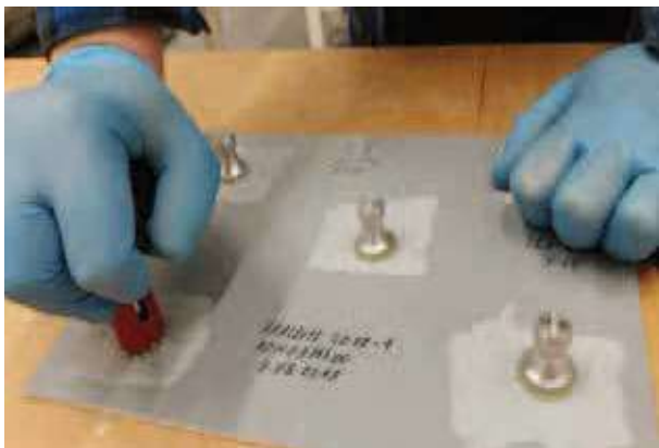
Fig. 1. Removing adhesive outflows Rys. 1. Usuwanie nadmiaru kleju
