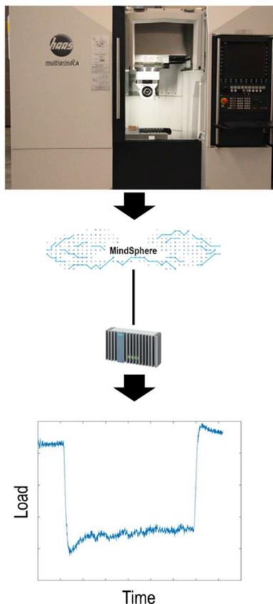
Fig. 9. In Situ measurement of load using Edge-Box
