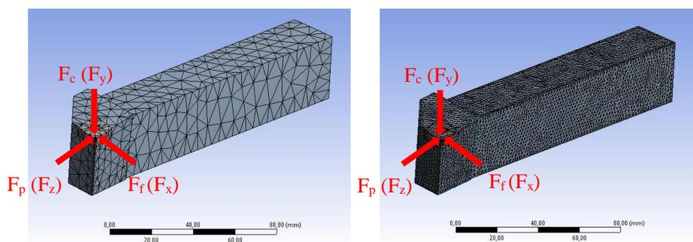
Fig. 7. Spreading of FEM mesh over the rectangular cutting tool (5mm-left, 1mm-right)
