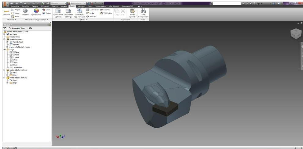
Fig. 6. 3D model of CAPTO tool holder prepared in Autodesk Inventor
