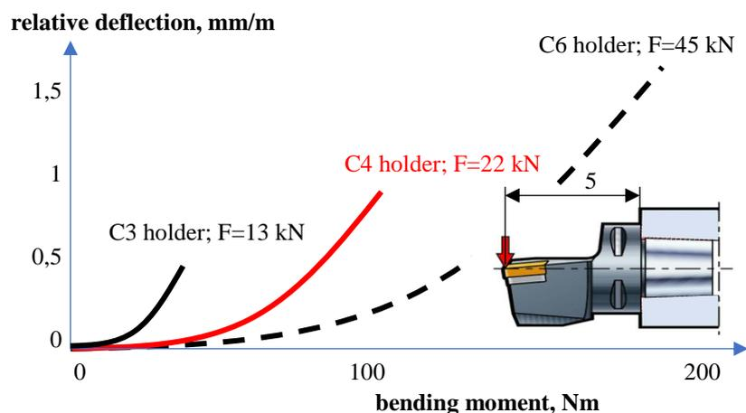
Fig. 2. Influence of selected polygonal shank tool holder on relative deflection of tool tip
