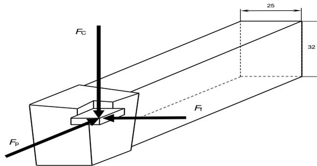
Fig. 4. Force components acting on rectangular shank turning tool
