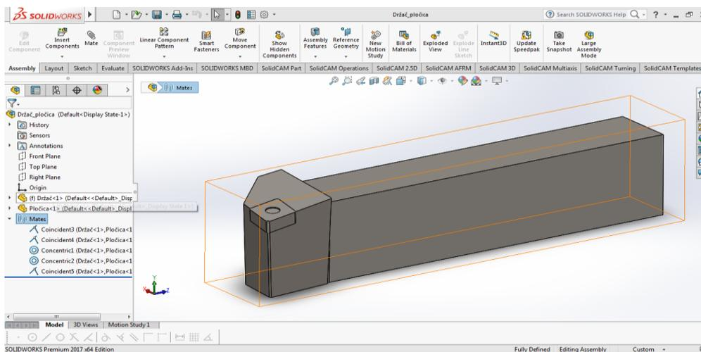
Fig. 5. Model of cutting tool holder with insert
