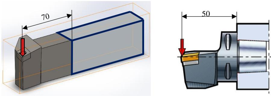
Fig. 1. Functional length of tool holders
