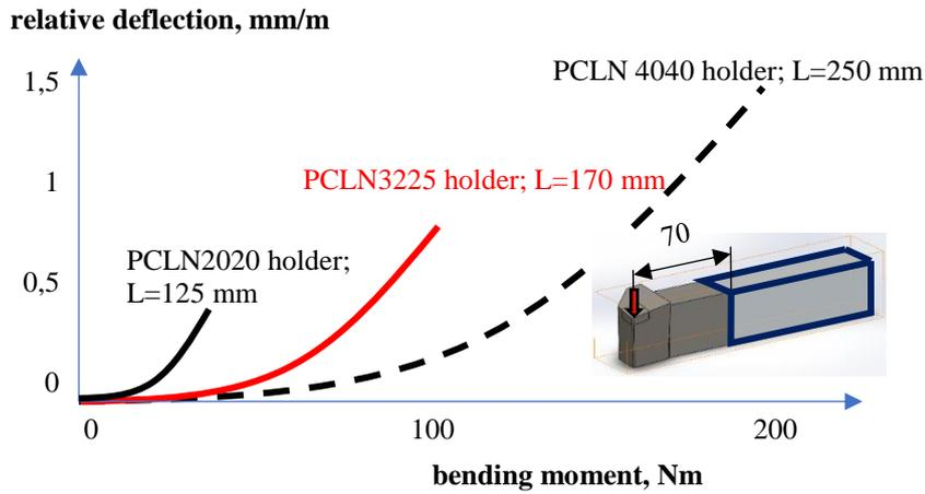
Fig. 3. Influence of selected rectangular shank tool holder on relative deflection of tool tip
