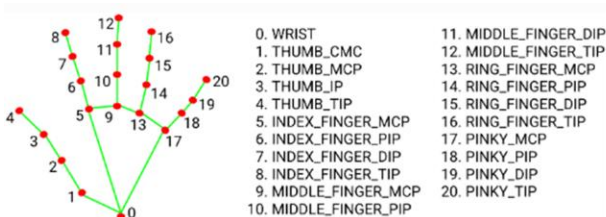
Fig. 1. The 21 critical points of a palm detected by MediaPipe Hands (MediaPipe, online)
