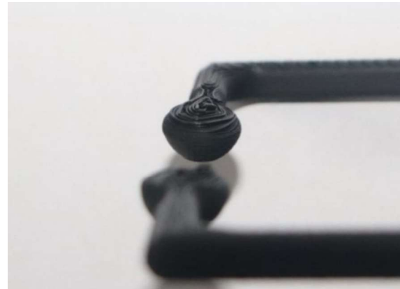
Fig. 5. Printing defect of spherical elements
