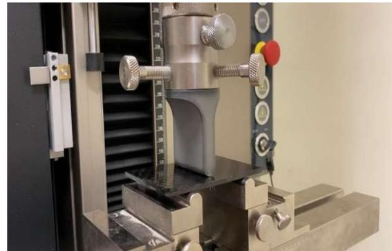
Fig. 10. Bending flexural strength test
