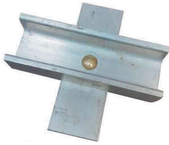
Fig. 3. Sample for testing the tensile strength of rivet heads
