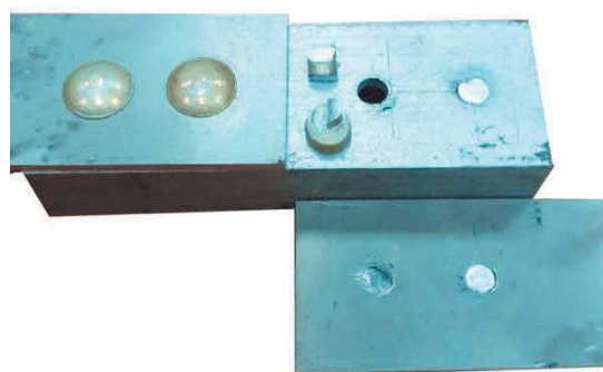
Fig. 13. Nature of fatigue failure of rivets of a single-strap sample with C-profile
