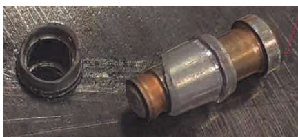
Fig. 6. Destruction of Huck rivet in an attempt to detach the head
