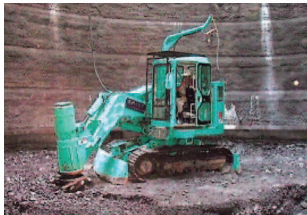
Rys. 2. Koparka do szybów Kayaba System Machinery Co., Ltd. [5] Fig. 2. Shaft excavator Kayaba System Machinery Co., Ltd. [5]
