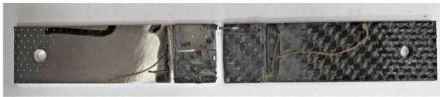
Fig. 5. The specimen after the strength test
