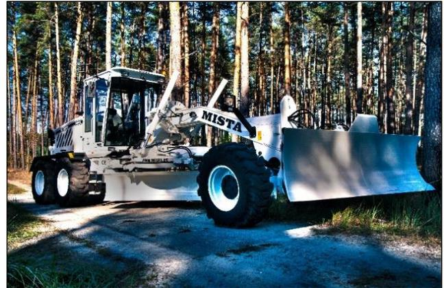
Fig. 1. Front view of the Mista RD-165 FHAD grader
