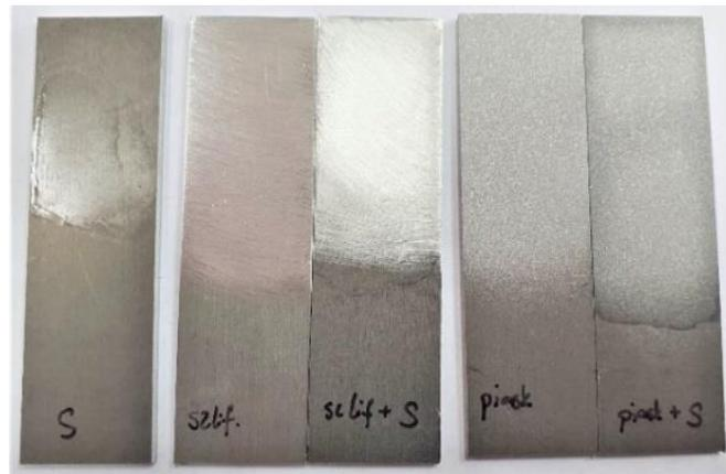
Fig. 8. Surface roughness test specimens prepared by the following methods (from left): primer, grinded, grinded + primer, sanded, sanded + primer
