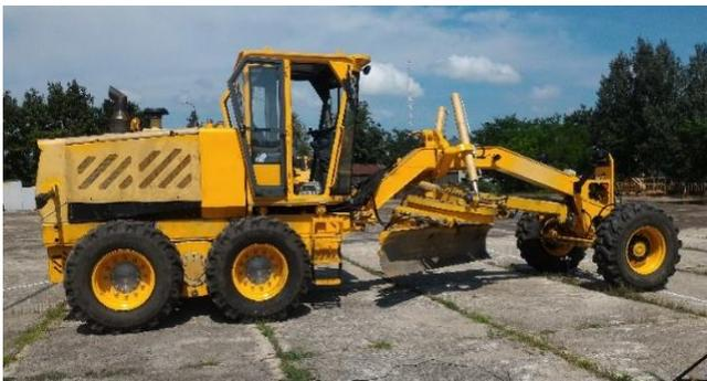
Fig. 4. MISTA RD-165 FHAD – first tested prototype
