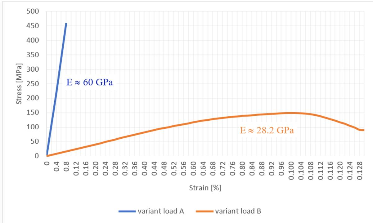
Fig. 8. Curves  $\sigma = \sigma(\varepsilon)$  of composite No. 1
