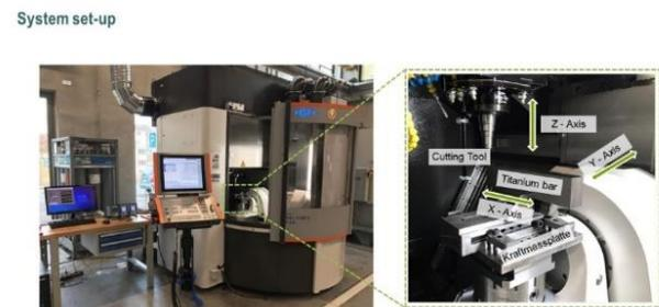
**Fig. 10.** Experimental setup of cryogenic milling of titanium
