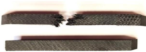
**Fig. 12.** Destruction of composite No. 3 in variant B
