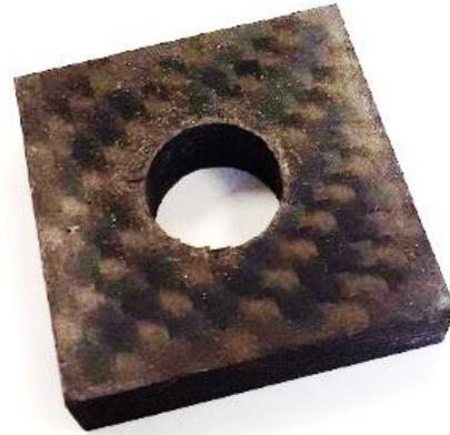
Fig. 6. Cube cut out of 7.3 mm thick composite
