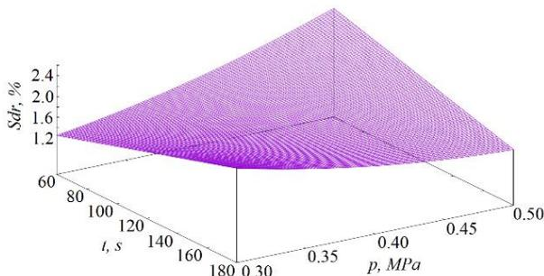
**Fig. 8.** Graph showing the influence of time  $t$  and pressure  $p$  on the value of the roughness parameter  $Sdr$  ( $d = 1$  mm)
