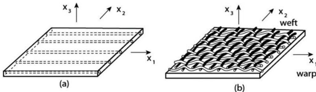
Fig. 2. Directions of orthotropy of the composite reinforced: a) unidirectional, b) fabric [3]
