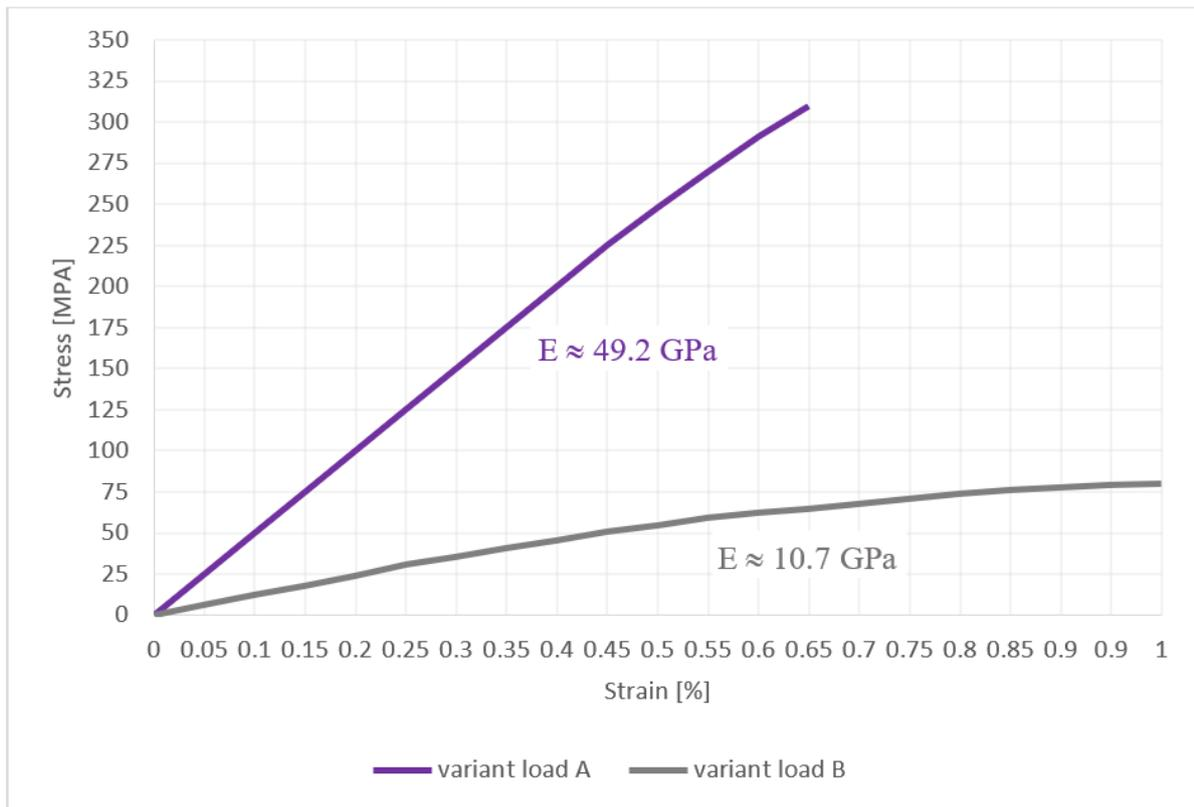
Fig. 10. Curves  $\sigma = \sigma(\epsilon)$  of composite No. 3
