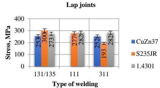
Fig. 4. Stress of lap welded joints
