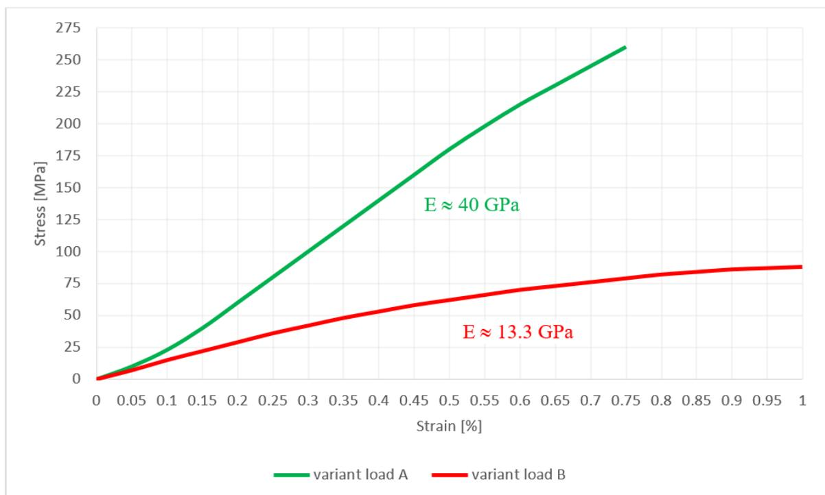
Fig. 9. Curves  $\sigma = \sigma(\varepsilon)$  of composite No. 2
