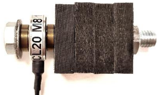
Fig. 4. Four composite cubes and a load cell bolted together with an M8 screw
