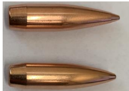
Fig. 2. Bullets used for the experiment: Top: secant ogive profile Lapua Scenar-L, Bottom: tangent ogive profile Lapua Scenar
