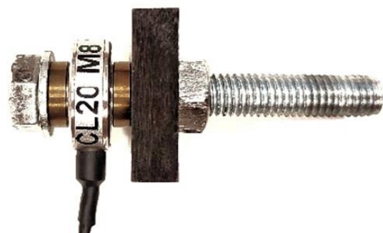
Fig. 5. One composite cube and force sensor bolted together with an M8 screw
