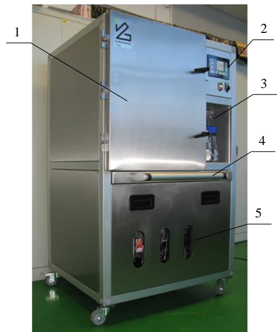
Fig. 8. Prototype of the test stand: 1 - emission chamber, 2 - control panel, 3 - air sampling port and water tank, 4 - pull-out shelf, 5 - air preparation module
