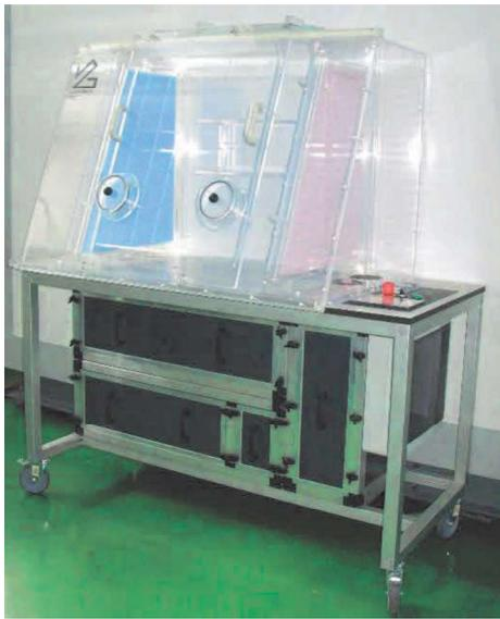
Fig. 6. Prototype laminar flow cabinet made of plastic
