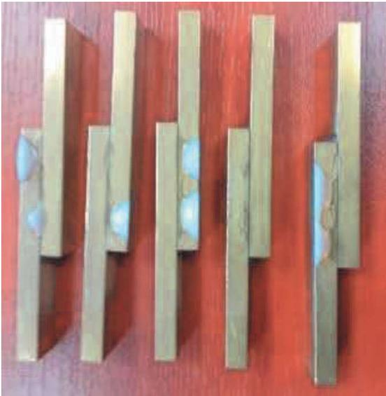
**Fig. 16.** A batch of brass samples bonded with Epidian 57 / Z1 adhesive
