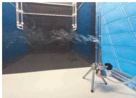
**Fig. 8.** Airflow smoke test
