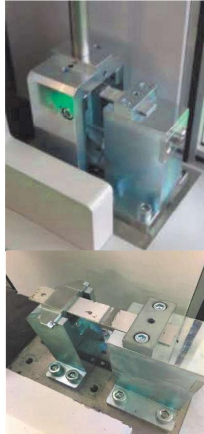
Fig. 8. The sample attached to the impact tests
