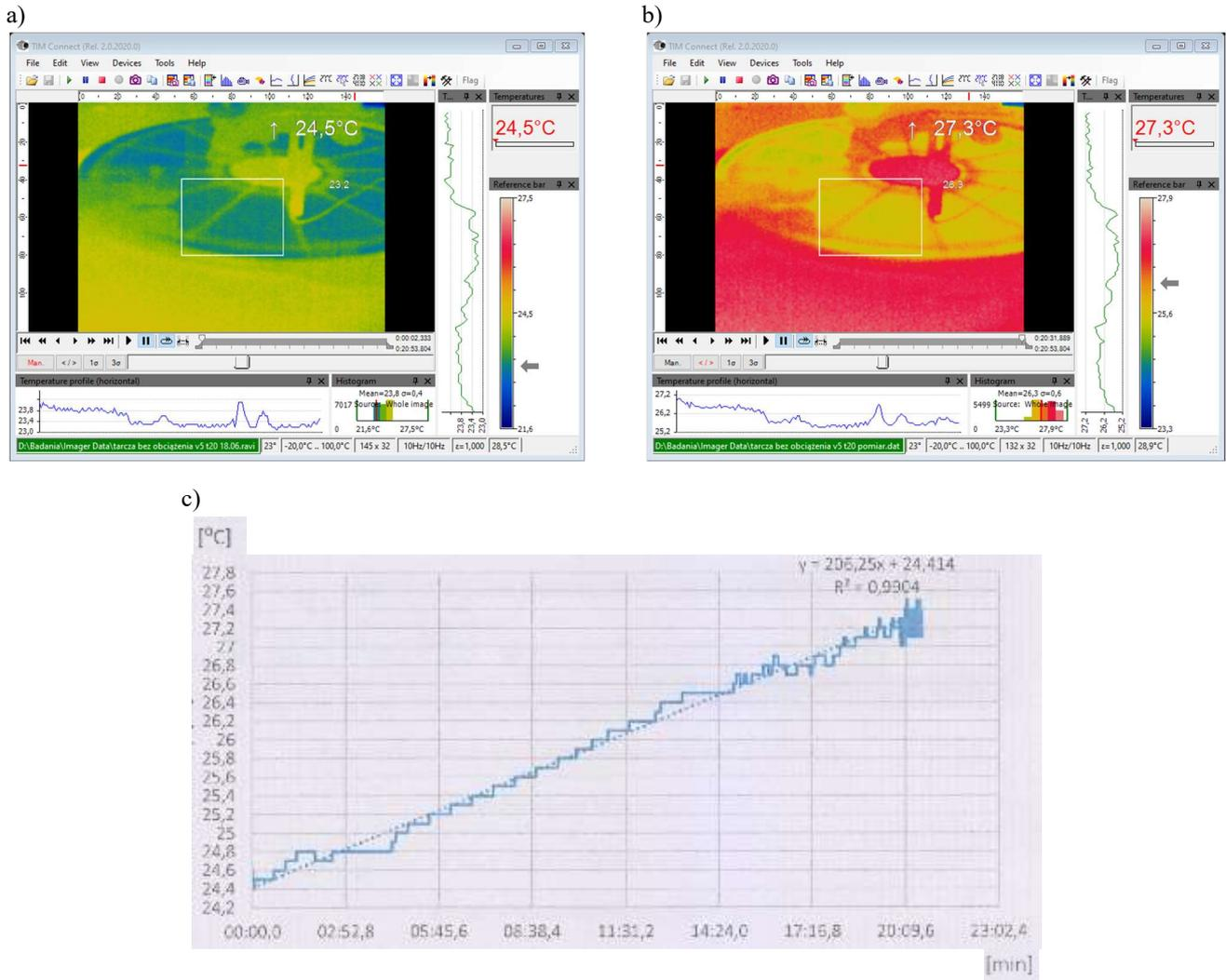
Fig. 7. Results of the measurements of the temperature of lapping disc in idle mode: a) in the initial moment, b) after 20 min ( $n = 40 \text{ min}^{-1}$ ), c) graph showing the increase of the temperature of the lapping disc in time (on average,  $0,14^\circ\text{C}/\text{min}$ )
