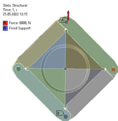
Fig. 9. The diagram of the boundary conditions of the FEM model
