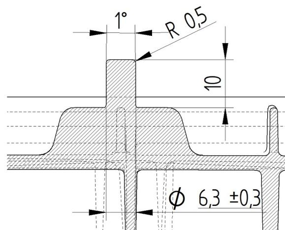
Fig. 2. Dimensions of an fixing pin
