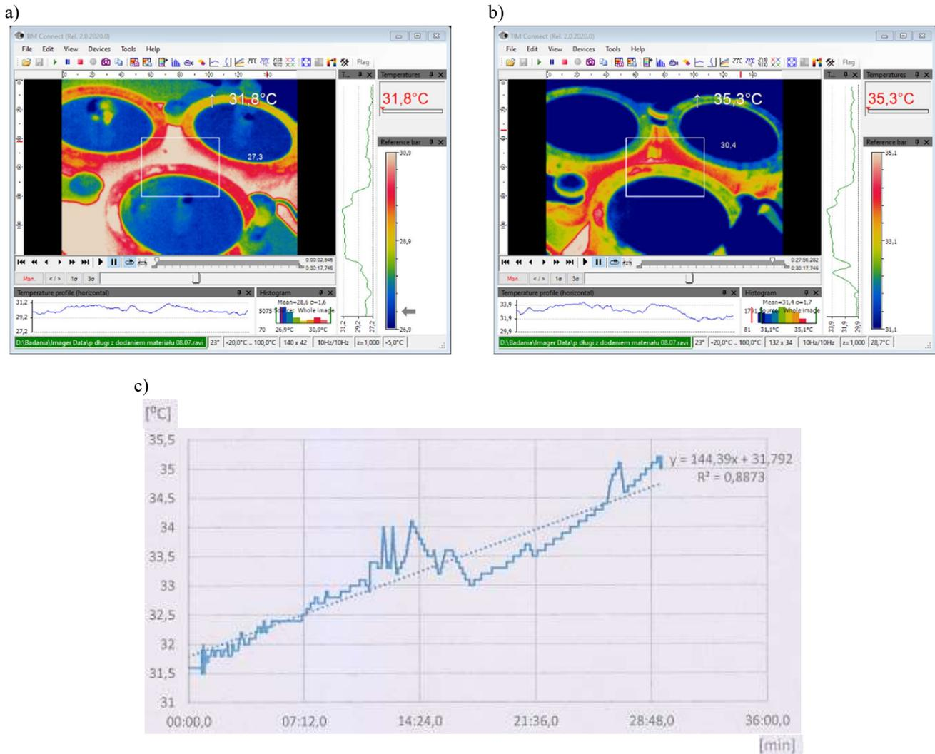
Fig. 12. Results of the measurements of the temperature of the actuating system during lapping of steel elements: a) in the initial moment, b) after 30 minutes ( $n_1 = 80 \text{ min}^{-1}$ ), c) graph showing the increase of temperature in time
