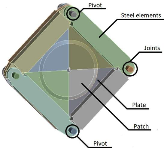
Fig. 4. Geometric model of the repaired plate with a frame
