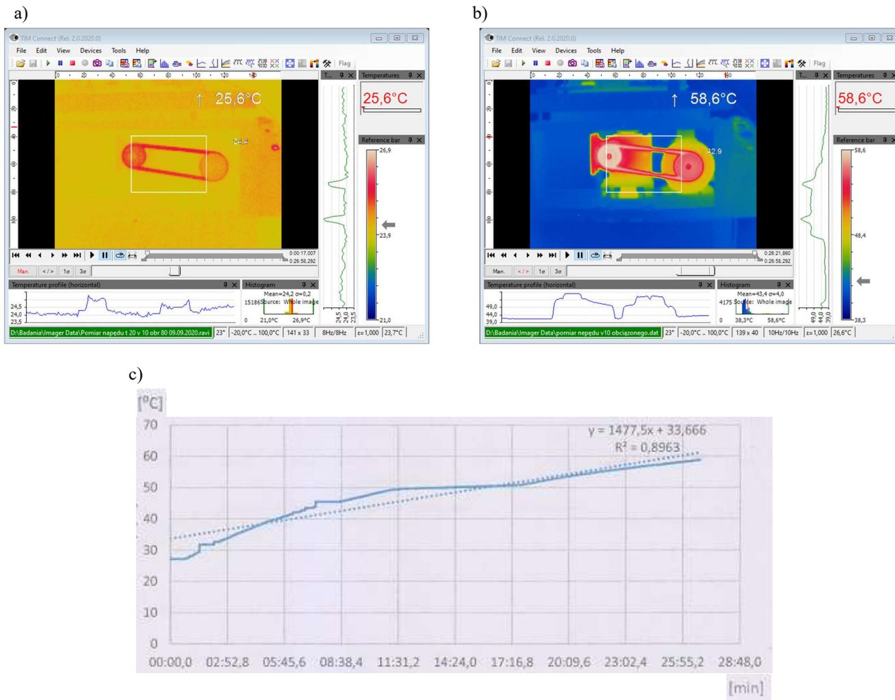
Fig. 6. Results of the measurement of the temperature of the lapping machine drive system: a) in the initial moment, b) after 20 min of dressing the lapping disc with guiding rings ( $n_t = 80 \text{ min}^{-1}$ ) and manual refilling of the abrasive after 11.5 min, c) graph presenting the increase of the temperature of the belt drive in time
