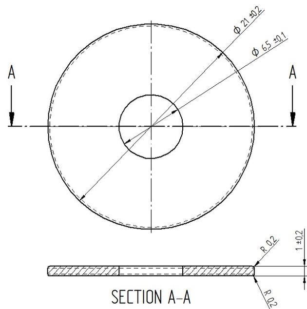
Fig. 1. Dimensioned drawing of a securing washer
