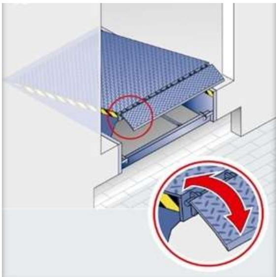
Fig. 1. Reloading ramp with a folding floor
