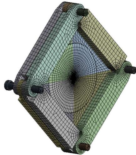
Fig. 6. The view of the model with the division into finite elements, the so-called mesh
