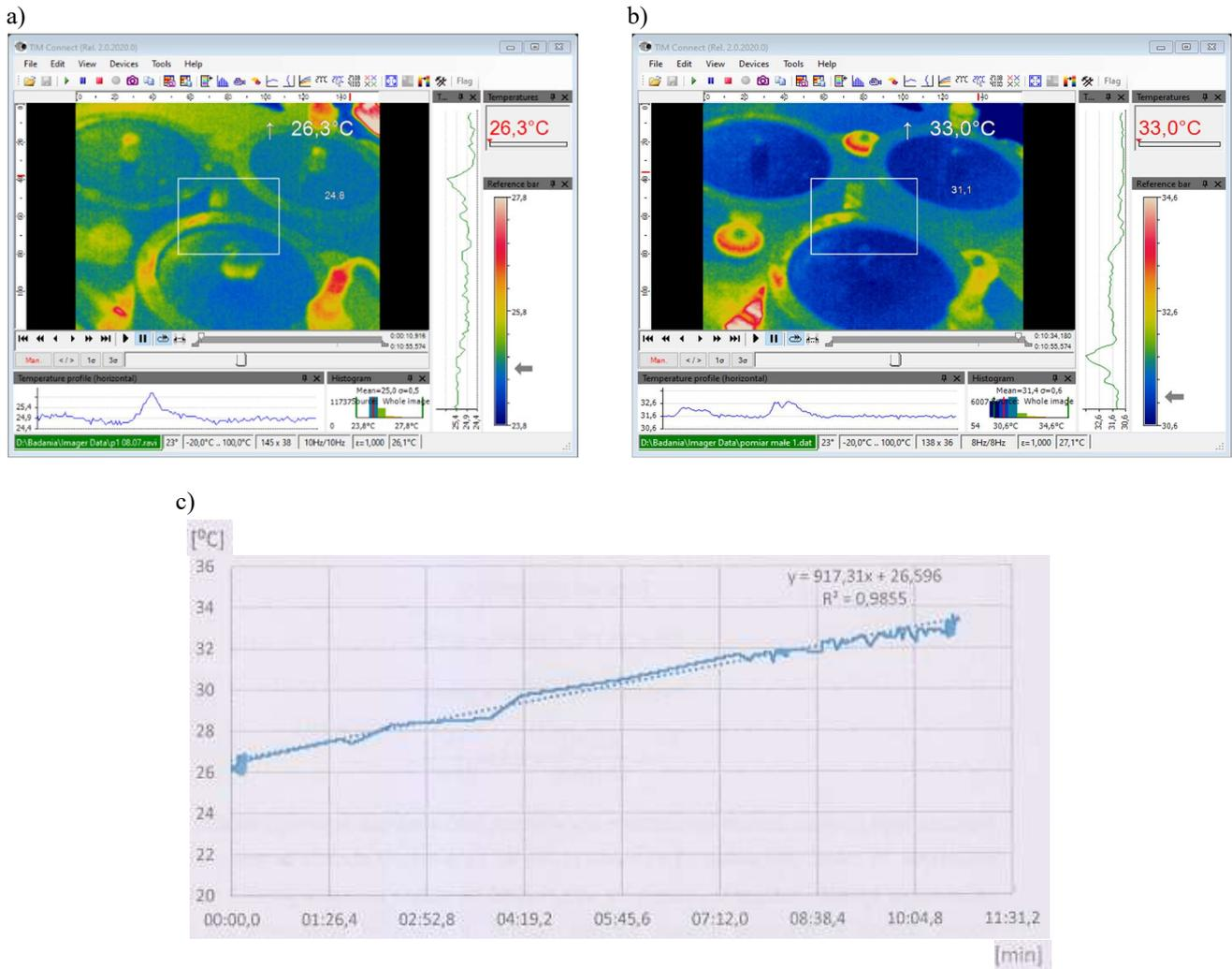
Fig. 9. Results of the measurements of the temperature of the actuating system during lapping of steel elements: a) in the initial moment, b) after 10 min ( $n_r = 80 \text{ min}^{-1}$ ), c) graph showing the increase of the temperature in time (on average by  $0.67^\circ\text{C}/\text{min}$ )
