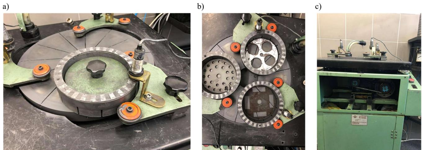
Fig. 2. View of: a) guiding ring containing machined elements and their ballast loads b) separators placed in the three guiding rings, c) uncovered drive system of Abralap 380 lapping machine
