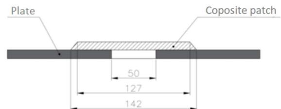
Fig. 3. The diagram of the repair node
