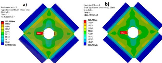
Fig. 14. Reduced stresses in the plate with the GFRP (a) and CFRP (b) patch
