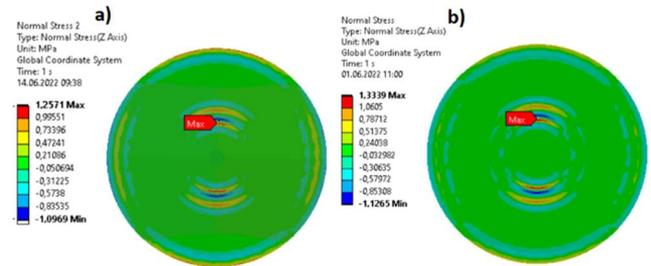
Fig. 15. Normal stresses to the adhesive surface for two patch variants: GFRP (a), CFRP (b)
