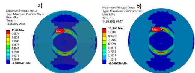
Fig. 16. Maximum main stresses in the adhesive layer for two patch variants: GFRP (a), CFRP (b)
