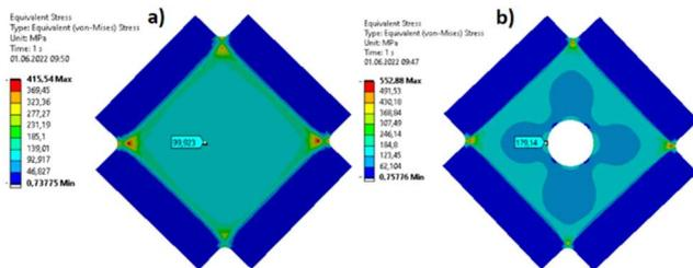
Fig. 13. Reduced stresses in the plate for undamaged (a) and damaged (b)
