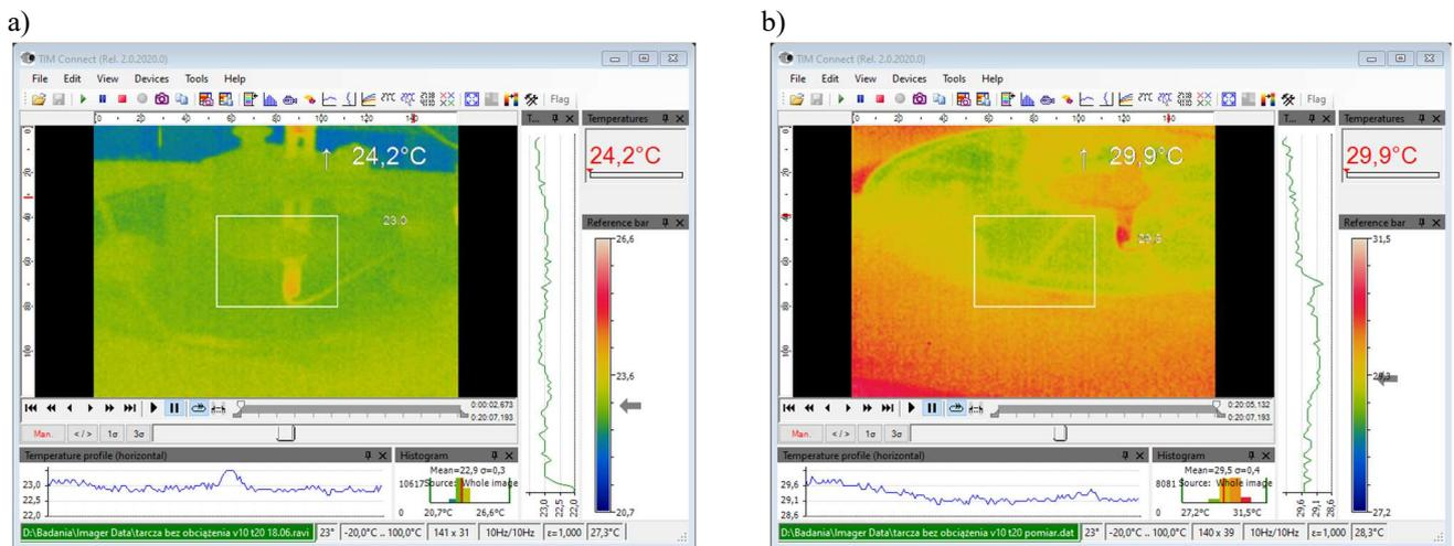
Fig. 8. Results of the measurements of the temperature of the lapping disc in idle mode: a) in the initial moment, b) after 20 minutes ( $n = 80 \text{ min}^{-1}$ )
