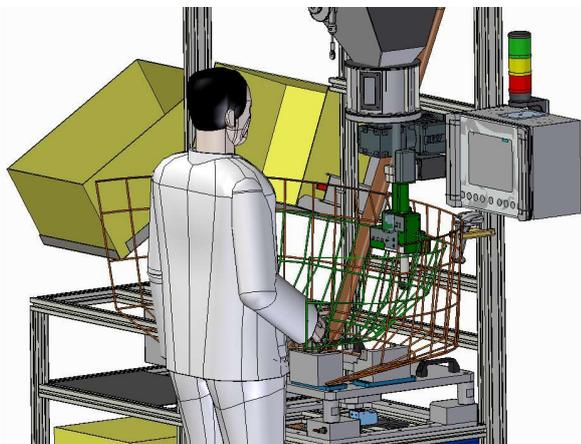
Fig. 7. Analysis of compliance with ergonomic conditions
