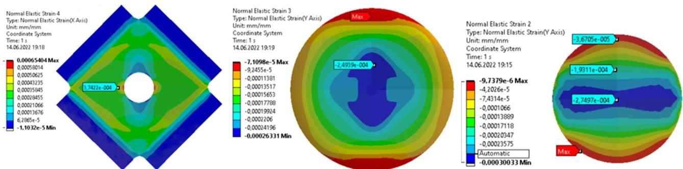
Fig. 12. Deformation values for the plate, glass fiber patch and reinforcement insert
