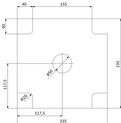
Fig. 1. Dimensions and shape of the plate used in the test
