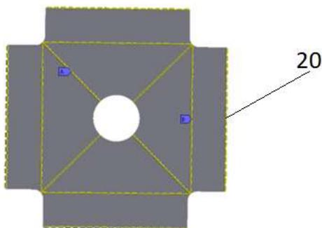
Fig. 5. Scheme of division of the slab model into 8 geometric elements
