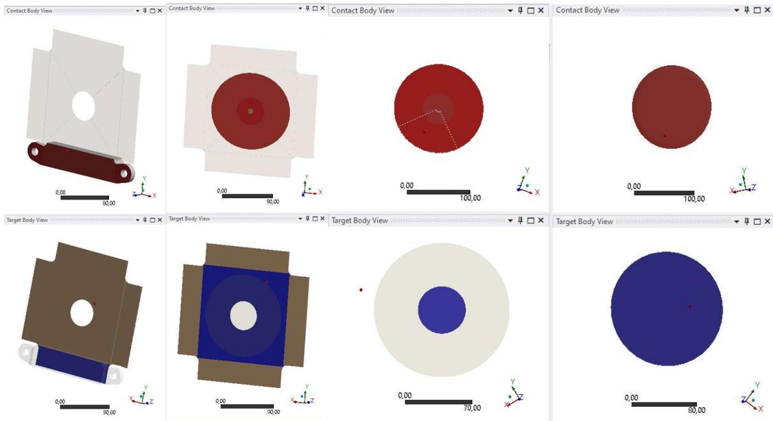
Fig. 7. Bonded contacts between the individual elements (red and purple indicate the contact area), from the left, the frame with the plate, the adhesive layer with the plate, the adhesive layer with the insert and the adhesive layer with the patch
