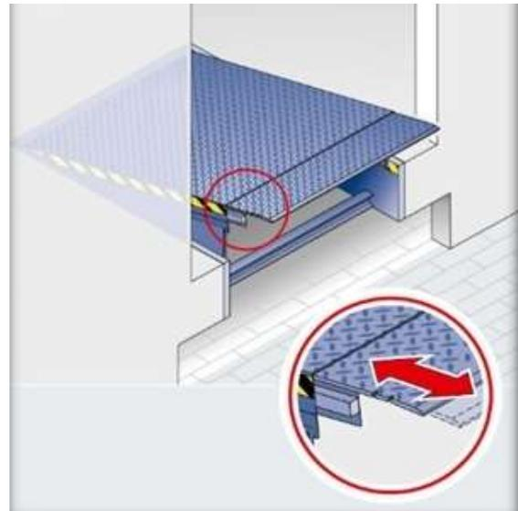
Fig. 2. Reloading ramp with a sliding floor
