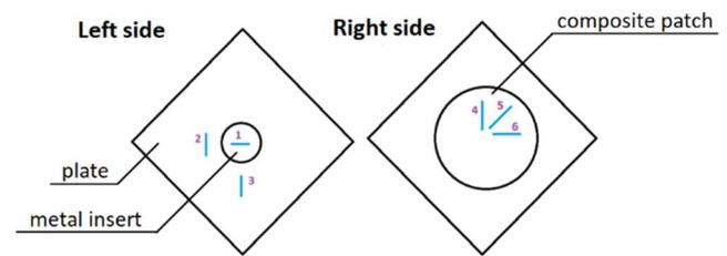
Fig. 11. Distribution and numbering of strain gauges mounted on the specimen
