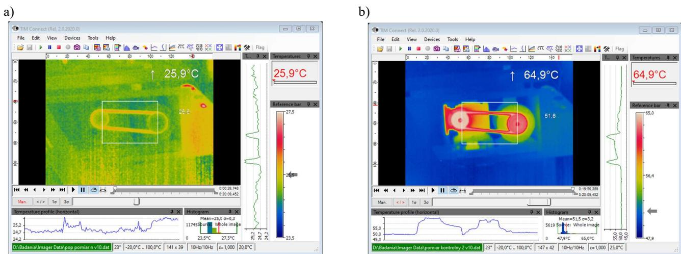
Fig. 4. Results of the measurements of the temperature of the drive system of the lapping machine: a) in the initial moment, b) after 20 minutes, without guiding rings placed on the lapping disc ( $n_t = 80 \text{ min}^{-1}$ )
