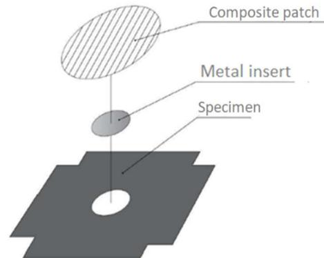
Fig. 2. Elements of the repair node
