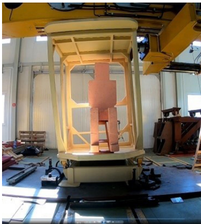
Fig. 19. ROPS structure under the lateral load
